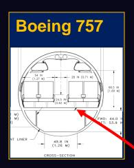
Most of the Structure is in Lower 1/3 of the airframe
